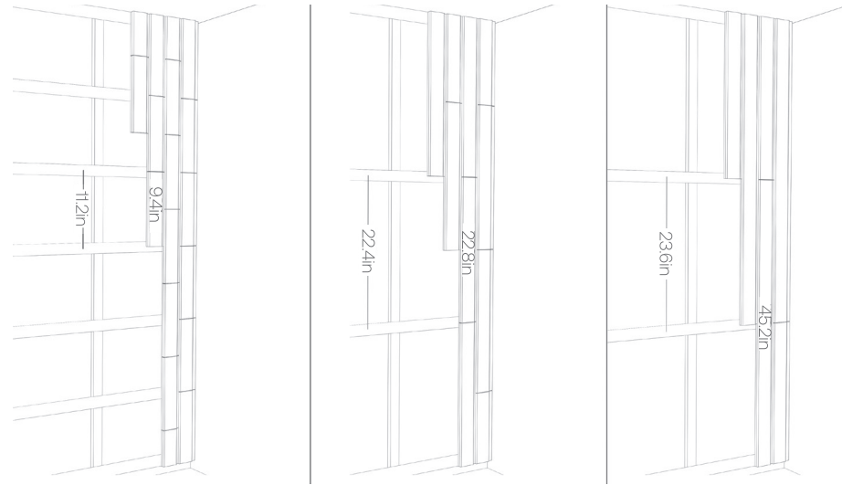
Tiles by Thermory paneling vertical installation
