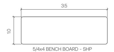
Profile Type: Sizing: Installation: Scale: Thermo-Spruce Bench Board 5/4x4 BENCH BOARD - SHP 40mm FG Screw 1'-o" = 1'-o"
