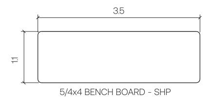
Profile Type: Sizing: Installation: Scale: Alder or Aspen Bench Board 5/4x4 BENCH BOARD - SHP 40mm FG Screw 1'-o" = 1'-o"
